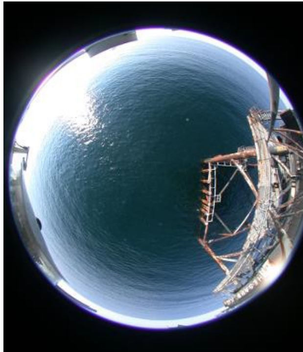
Figure 1: Fish-eye photograph taken near the end of the 8-meter boom where the upwelling pyrgometer was installed. The right side of the picture shows the lighthouse legs/structure occupying a significant portion of the static pyrgometer field of view.
