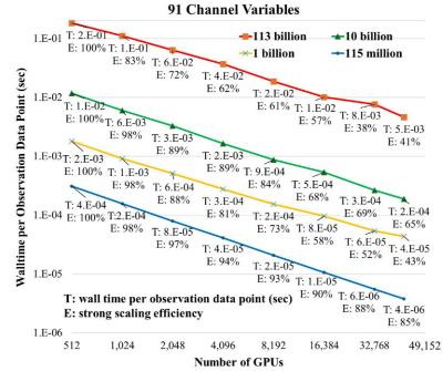
ORBIT achieves 1.6 exaflop sustained computing throughput on 6,144 Frontier nodes (49,152 GPUs), with strong scaling efficiency between 44% to 85% for model sizes of 100M, 1B, 10B, and 113B.
