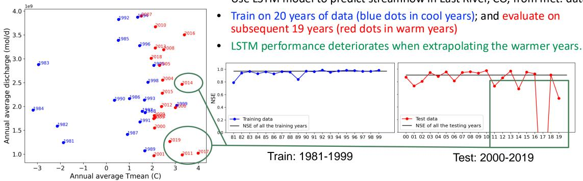
Use LSTM model to predict streamflow in East River, CO, from met. data. •
