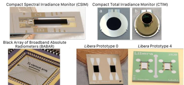
**Figure 4.** VACNT ESRs for ERB measurements
