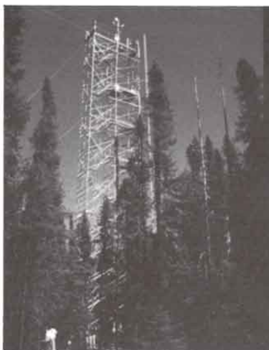
Double-scaffold flux measurement tower at the Old Black Spruce site in the BOREAS Southern Study Area.
