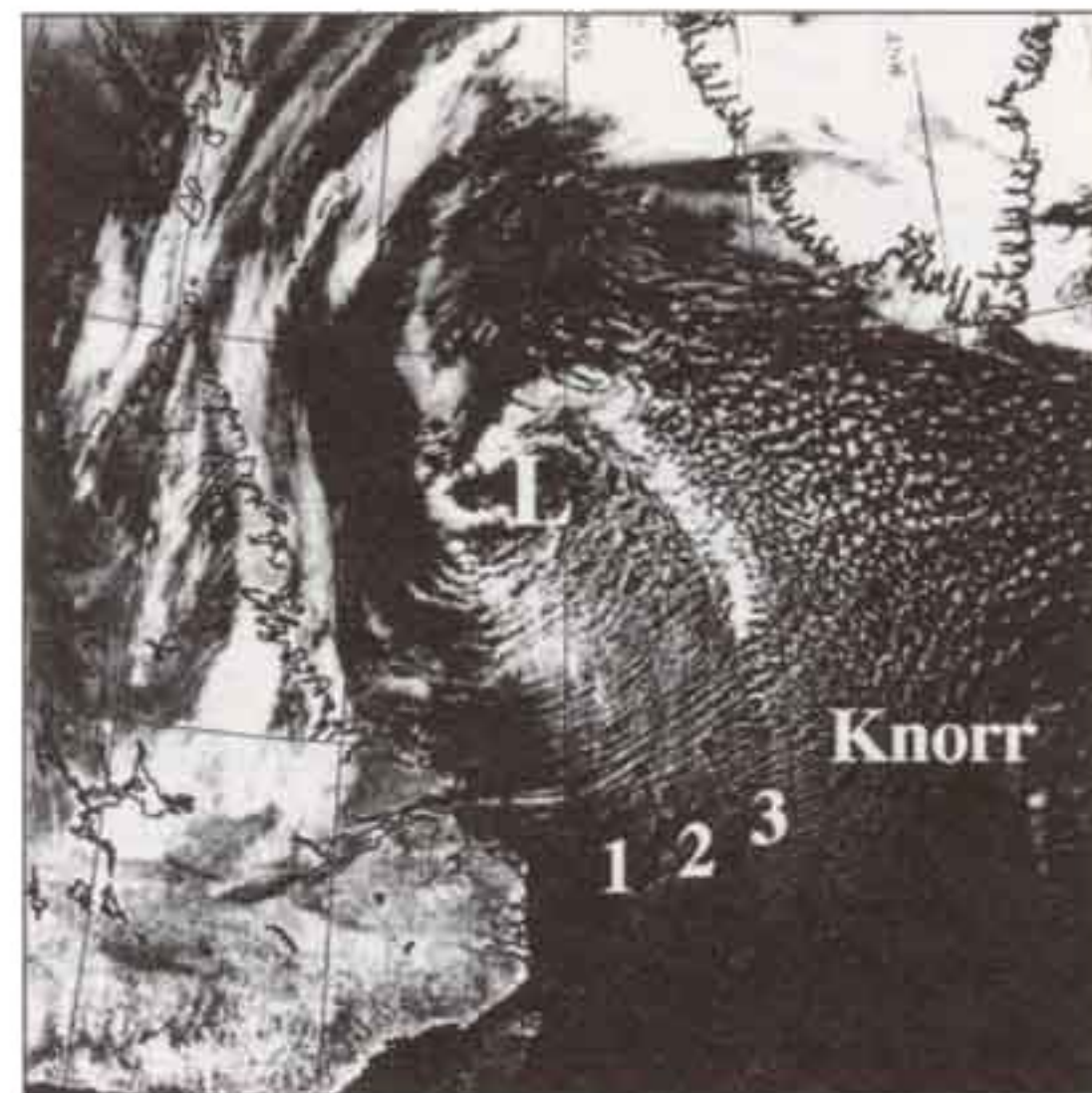
Figure 1: NOAA AVHRR Infrared Satellite Image at 11:19 GMT on February 8, 1997, showing an extratropical cyclone over the Labrador Sea. An aircraft mission was flown on this day to investigate the structure of the linear cloud bands over the Labrador Sea and to measure the exchange of heat across the air-sea interface. The three low-level stacks (1,2,3) that were flown are indicated. Also shown is the 12 GMT position of the RV Knorr.
